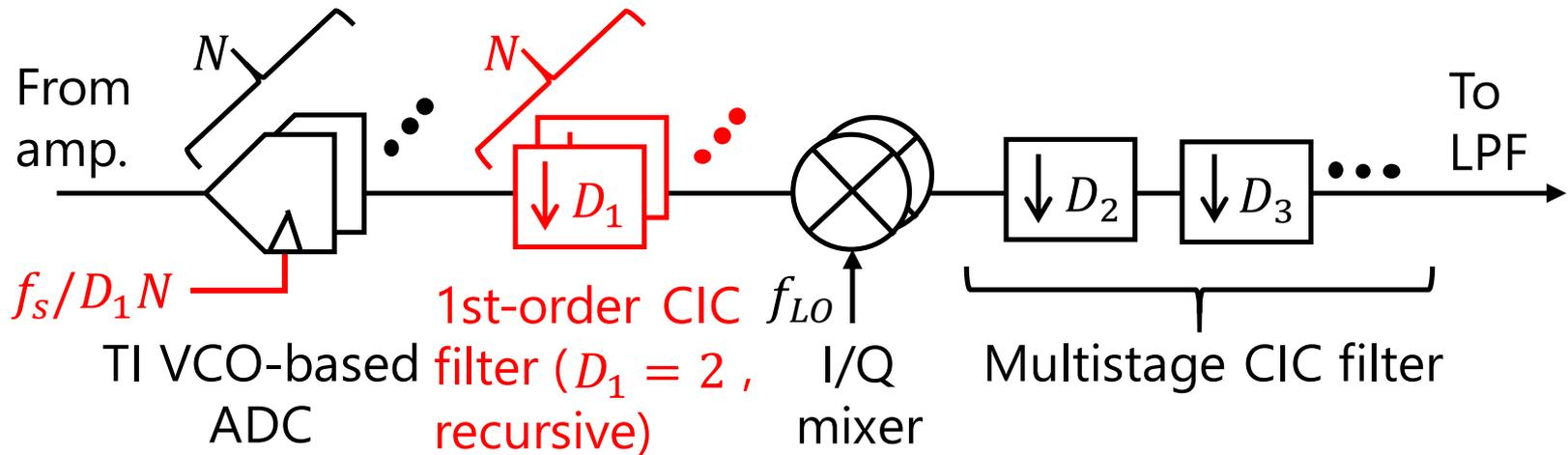
1. Place first-order recursive CIC filters with  $D_1 = 2$  after a TI VCO-based ADC:
