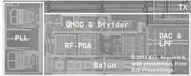
**Fig. 8** Microphotograph of the fabricated transmitter.
