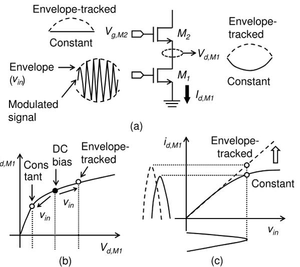
**Fig. 5** Concept of envelope-tracked biasing: (a) Transconductor with envelope-tracked or constant biasing, (b)  $I_{d,M1}$  versus  $V_{d,M1}$ , and (c)  $i_{d,M1}$  versus  $v_{in}$ .
