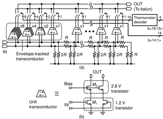
**Fig. 4** (a) Block diagram of the RF-PGA and (b) schematic of the transconductor.
