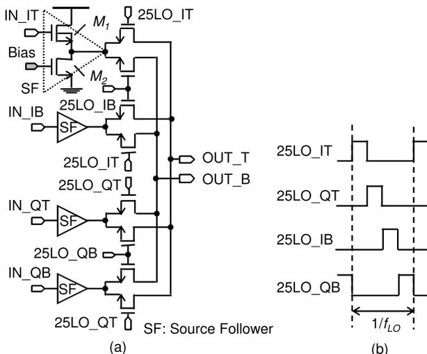
**Fig. 2** (a) Schematic of the proposed QMOD and (b) the waveform of 25%LO signals.
