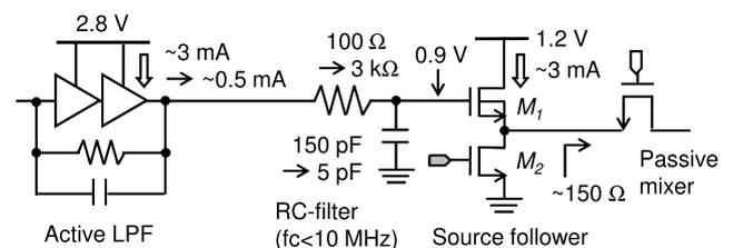
**Fig. 3** Proposed driver stage for the passive mixer.
